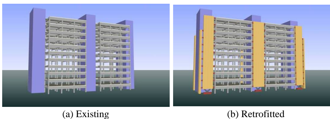
Figure 6. 3D view of G3 Building before and after retrofit
